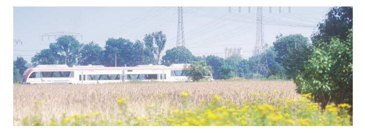
Optimal energy consumption values are achieved by the lightweight design: The ITINO's power weight is approximately 12 kW/t (operating weight at 50 % capacity). Noise emission is reduced to a minimum by noise protection measures and motor containment, thus enabling night-time operations even in urban areas.
